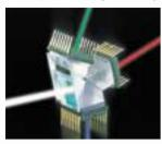
Panasonic designed the AG-DVX100B to deliver the highest sensitivity and picture quality in its class. At its heart is a 3CCD RGB system comprising three 1/3-inch, 470,000-pixel progressive CCDs developed especially for broadcast and professional applications. The new on-chip lens design achieves
